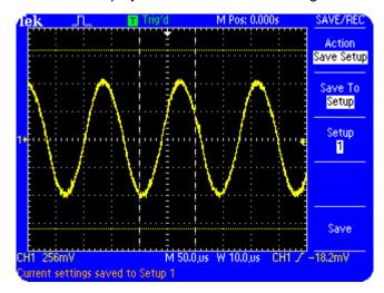
Figure 6.14: Saving an instrument setup
