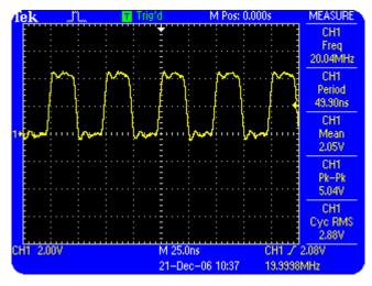
Figure 6.13a: Square waveform with five automatic measurements
