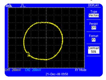
Figure 6.8: XY Display of two sine waves with 90° phase shift
