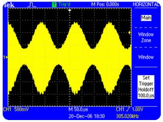
Figure 5.12: Stable AM signal using trigger holdoff
