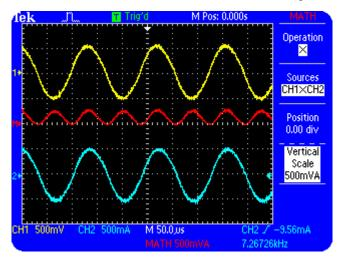
Figure 3.6: Display of CH1xCH2
