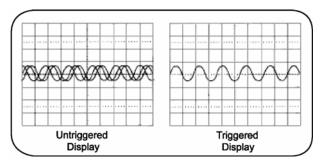
Figure 1.4: Untriggered and triggered display
