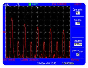
Figure 3.7: FFT display of the calibrator signal
