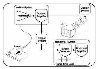
Figure 1.3: Block diagram of an analog oscilloscope
