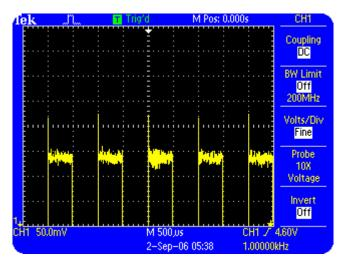
Figure 3.3: Vertical display, with 100 divisions of offset
