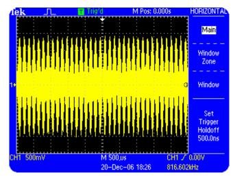
Figure 5.11: Complex AM signal without holdoff
