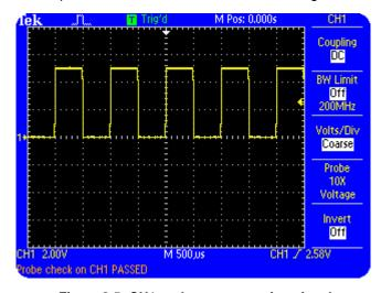
Figure 2.5: CH1 probe compensation signal
