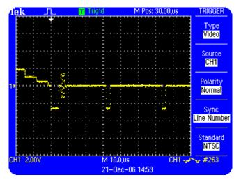
Figure 2.14c: Triggering on video lines
