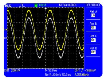
Figure 6.15: Saved and updating waveforms displayed
