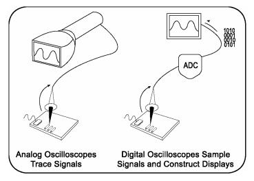
Figure 1.2: Analog and digital oscilloscopes
