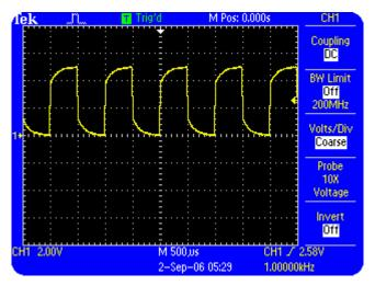
Figure 2.6: Probe undercompensated
