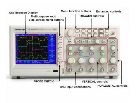
Figure 2.2: The TDS2024B digital storage oscilloscope
