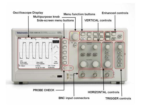
Figure 2.1: The TDS1001B digital storage oscilloscope
