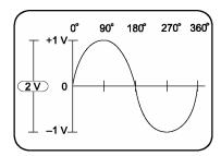
Figure 1.13: Phase in a sine wave
