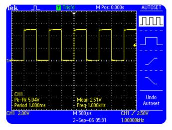
Figure 4.2: TDS2000B horizontal setup
