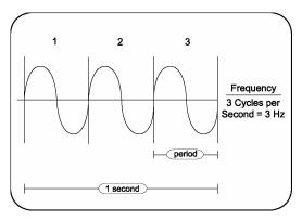
Figure 1.12: Frequency and period of a sine wave
