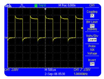
Figure 2.7: Probe overcompensated
