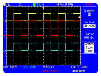
Figure 3.4:Display of CH1+CH2
