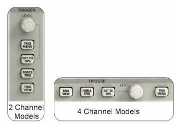
Figure 5.1: TRIGGER control sections
