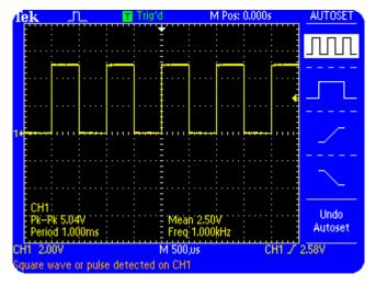
Figure 2.3: Square wave of 5 volts peak-to-peak at 1 kHz
