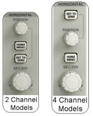
Figure 2.11: TDS1012B and TDS2024B HORIZONTAL controls
