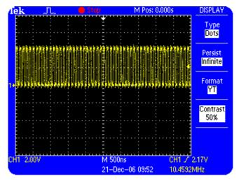
Figure 6.6: A noisy signal with infinite persistence
