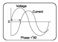
Figure 1.14: Phase shift between two sine waves
