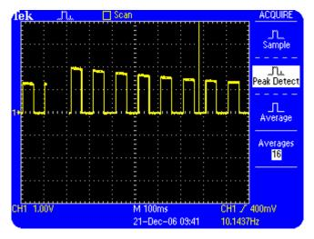
Figure 6.2: A noisy variable amplitude signal with glitches acquired with the Peak detect and scan display modes
