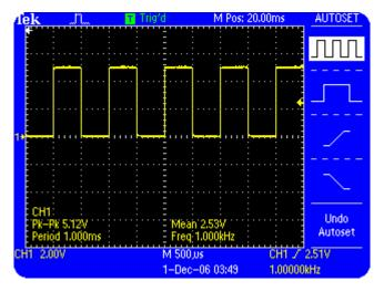
Figure 4.3: Delayed trigger position for a waveform
