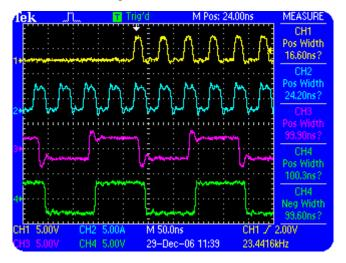
Figure 6.13b: Multiple Signals with the Same Measurements
